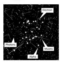
Illustration of particle tracking capability of Timepix3 device: The tracks of different particles of radiation background were recorded during 10 minutes in office space in Prague. Brightness corresponds to energy. No noise (clean zero) is seen in dark regions. All basic particle track types are seen nicely: muons = straight lines, alpha particles = bright balls, electrons = curving lines, gamma and X-rays = dots and blobs.
